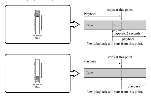
Set the REVERSE TIME control to the desired position and keep the right side of the pedal of the supplied foot control unit depressed to play back the tape.
